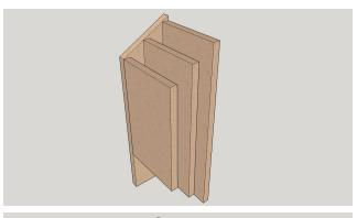
4. Line up the 1 x 8 x 16" cedar board in the center of the 1 x 6 board. Predrill holes for 1 %" nails and attach the two boards.
