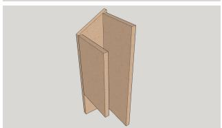
3. Line up the 1 x 8 x 12" cedar board along the shortest edge of the 1 x 6 board. Predrill holes for 1 %" nails and attach the two boards.
