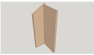
2. Line up the 1 x 8 x 20" cedar board along the longest edge of the 1 x 6 board. Predrill holes for 1 %" nails and attach the two boards.
