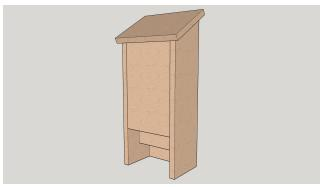
6. Line up the 1 x 8 x 10" roof piece on top of the angled end. Predrill holes and attach with nails.
