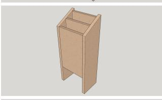
5. Predrill holes and attach the other 1 x 6 board with nails.
